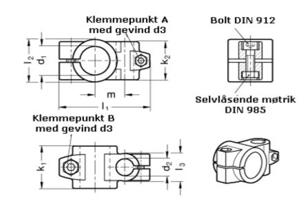
Adjustable clamp lever for d3 = GN 911-M 8-32 have to be ordred separately |1 = 81.5Adjustable clamp lever for d4 = GN 911-M 6-25 have to be ordred separately
